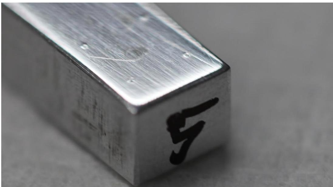
**Figure A.16:** Photo of the prepared sample before analysis: The deposited sample material is visible as darker area in the middle of the four orientation marks on the sample holder.
