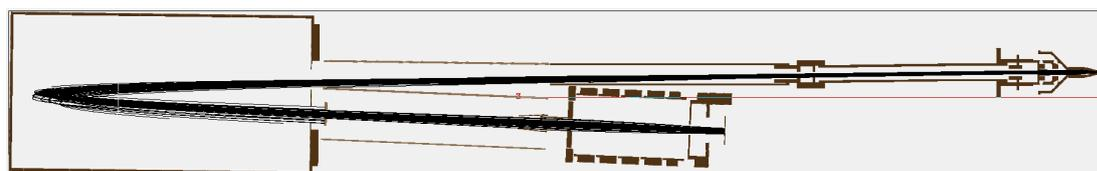
**Figure 4.9:** Simulated ion trajectories through the mass analyzer: The drawing shows a cross section of the mass analyzer in SIMION 8.1 with trajectories of 10.000 sample ions.
