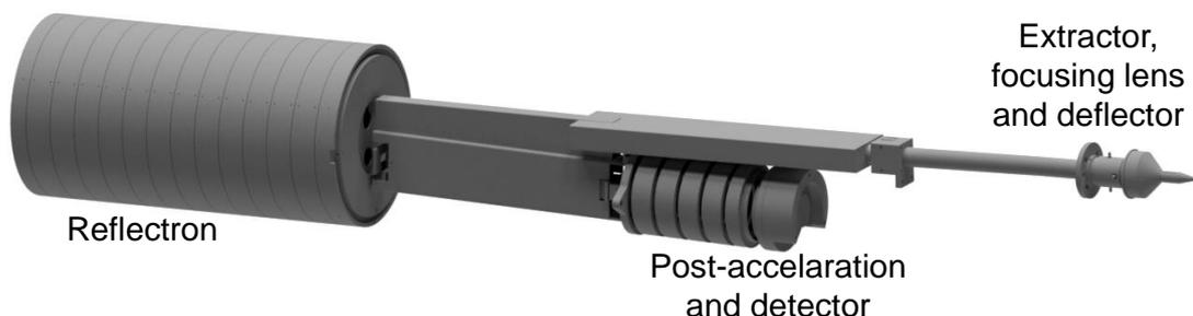
**Figure 4.7:** 3D representation of the TOF mass analyzer (simplified) including the main ion optical components based on the technical drawings and created by "Autodesk Inventor 2014".
