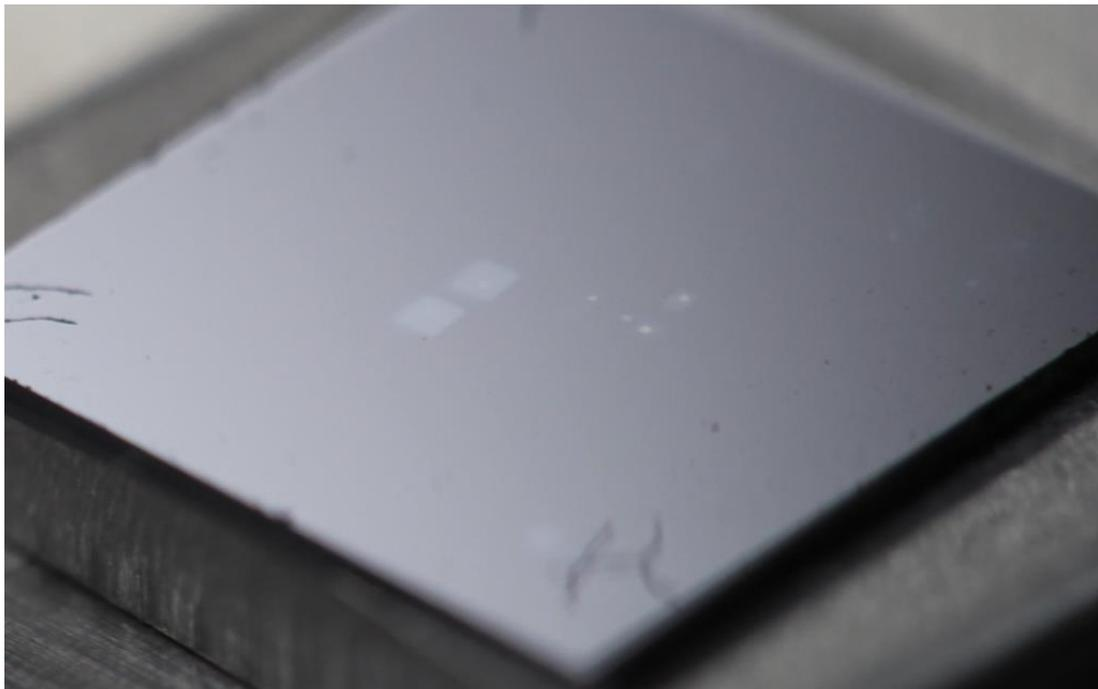
**Figure A.17:** Photo of the uranium particle containing silicon waver: The brighter fields in the middle are the analyzed areas. The two areas of  $500\ \mu\text{m} \times 500\ \mu\text{m}$  visible on the left side were used for test measurements. The four small areas on the right side mark the positions of the efficiency measurements. (one measurement was incomplete due to technical problems)
