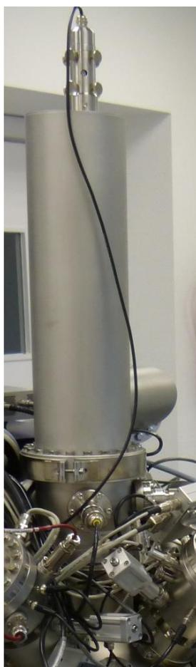
**Figure A.9:** Photo of the time-of-flight mass analyzer
